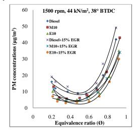
Fig. 10, equivalence ratio effect on PM concentrations with and without EGR for tested blends
