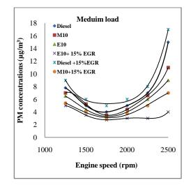
Fig. 7, Engine speed with medium load effect on PM concentrations with and without EGR for tested blends
