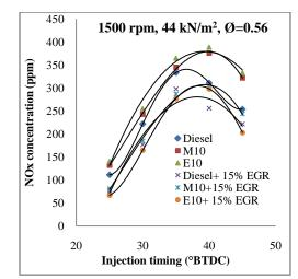
Fig. 11, injection timing effect on NOx concentrations with and without EGR for tested blends
