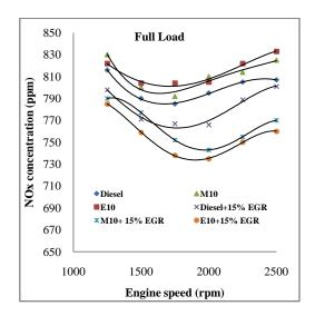
Fig. 5, Engine speed with full load effect on NOx concentrations with and without EGR for tested blends
