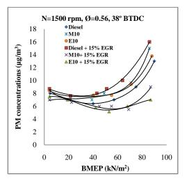
Fig. 2, load effect on PM concentrations with and without EGR for tested blends
