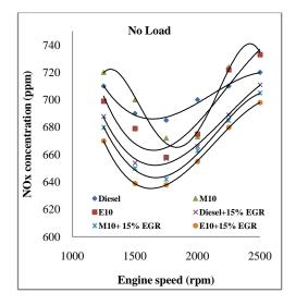
Fig. 3, Engine speed with no load effect on NOx concentrations with and without EGR for tested blends
