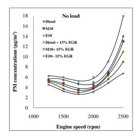
Fig. 6, Engine speed with no load effect on PM concentrations with and without EGR for tested blends
