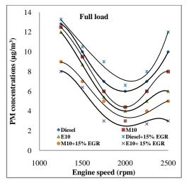
Fig. 8, Engine speed with full load effect on PM concentrations with and without EGR for tested blends
