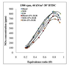
Fig. 9, equivalence ratio effect on NOx concentrations with and without EGR for tested blends
