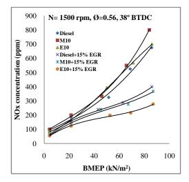
Fig. 1, load effect on NOx concentrations with and without EGR for tested blends
