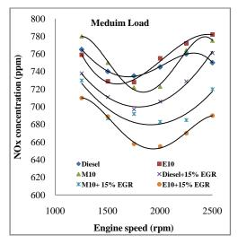
Fig. 4, Engine speed with medium load effect on NOx concentrations with and without EGR for tested blends
