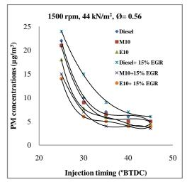
Fig. 12, injection timing effect on PM concentrations with and without EGR for tested blends
